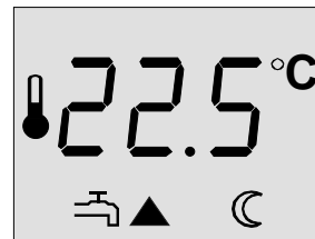
Display in energy saving mode Heating ON DHW ON
