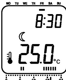
The Digital Thermostat is a weekly programmable thermostat, with 7 day/24 hour programs that can be set as required. For each hour you can set the Digital Thermostat so that either the CT (COMFORT) or (EVENING) temperature mode operates. The Digital Thermostat comes with a preinstalled program that will accommodate many users' requirements
