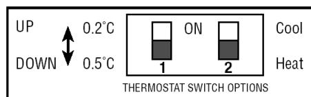
**DIP switch 1** adjusts the sensitivity of the thermostat. In the DOWN position if the temperature variation is greater than 0.5°C the thermostat is activated. In the UP position it will activate if the variation is greater than 0.2°C.
