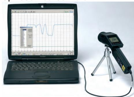
OptrisConnect oscilloscope software with 20 readings per second
