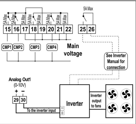
**Plant with 1 frequency compressor + 2 standard compressors and 2 fans:**
