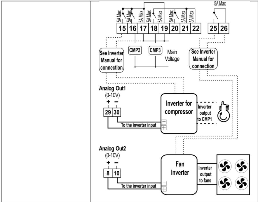
**Plant with 4 compressors with inverter for fans:**
