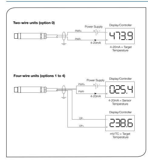
The PyroCouple Series is a range of high quality, low cost, compact sensors which measure the temperature of inaccessible or moving objects and materials. They measure temperatures from -20°C to 500°C, accurately and consistently, with an outstanding response time of 240 ms.
