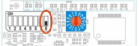
If terminal line resistance **has** to be connected (if MCM260 is the last device of the network), set last dip-switch as shown in figure below.
