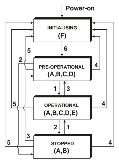
NMT services allow changing status nodes at any time. NMT message consists of CAN-header (COB-ID = 0) and 2 data bytes. One byte
