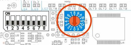
For both selectable protocols (Modbus or CANopen), rotary switch positions between 1 and 8 are **address offset multiplier**, while positions between 9 and F are **baud-rate**. Node address will be:
