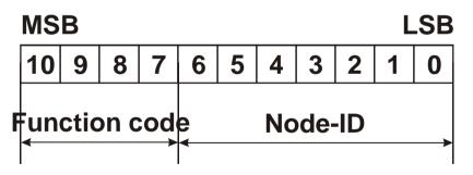
Pre-defined connection set defines 4 Rx PDOs, 4 TX PDOs, 1 SDO, 1 Emergency Object and 1 Node-Error-Control Identifier<sup>1</sup>. It also support broadcasting of non-confirmed NMT Module Control Services, SYNC and
