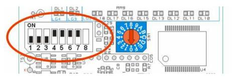
Subsequently procedure shown in the following page has to be done to configure address offset multiplier and baud-rate.
