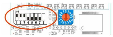
A CANopen network must have a  $120\Omega$  terminal line resistance. If more devices have to be connected in cascade, that resistance has to be connected to the last MCM260 of network, at the end of the line only.
