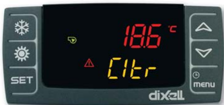
Each alarm has a dedicat label (eg. C1tr: thermal compressor 1 alarm)
