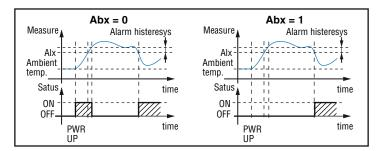
2. A "Latched alarm" (manual reset) is an alarm that will remain active even if the conditions that generated the alarm no longer persist. Alarm reset can be done only by an external command (U button, digital inputs or serial link).
