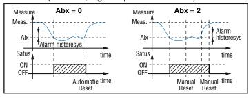
**3.** An "Acknowledgeable" alarm is an alarm that can be reset even if the conditions that generated the alarm are still present. Alarm acknowledge can be done only by an external command (U button, digital inputs or serial link).
