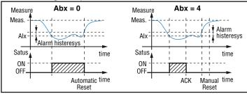
The instrument does not memorize in EEPROM the alarm status. For this reason, the alarm status will be lost if a power down occurs.
