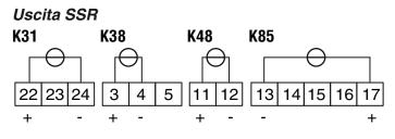
Logic level 0: Vout < 0.5 VDC; Logic level 1: 12 V ±20% @ 1 mA; 10 V ±20% @ 20 mA.
