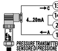
For linear signals 0/4..20 mA with two-wires sensors.
