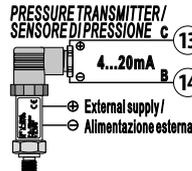
For linear signals 0/4..20 mA with external power supply for sensor.
