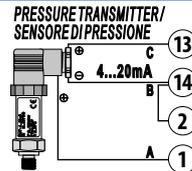
For linear signals 0/4..20 mA with three-wires sensors.
