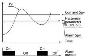
Lower deviation alarm value of alarm setpoint greater than "0" and hysteresis value greater than "0" (Par. 58  $R_{I.H.Y.} > 0$ ).\*\*\*
