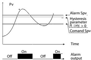
Upper deviation alarm value of alarm setpoint greater than "0" and hysteresis value greater than "0" (Par.58  $R_{I.H.Y.} > 0$ ).\*\*
