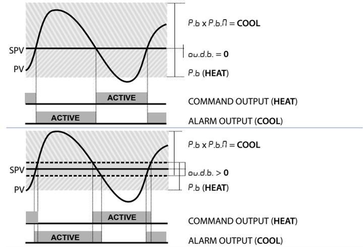
The parameter  $c.o.c.t.$  has the same meaning as the heating time cycle  $t_c$ . Par. 41  $c.o.o.f.$  (Cooling Fluid – word 2041) pre-selects the proportional band multiplier  $P_b, \bar{n}$ , and the cooling PID cycle time  $c.o.c.t.$ , basing on the type of cooling fluid:
