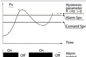
Lower deviation alarm value of alarm setpoint less than "0" and hysteresis value greater than "0" (Par. 58  $R_{I.H.Y.} > 0$ ).\*\*\*
