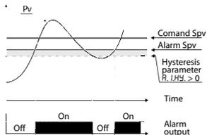
Upper deviation alarm value of alarm setpoint less than "0" and hysteresis value greater than "0" (Par.58  $R_{I.H.Y.} > 0$ ).\*\*
