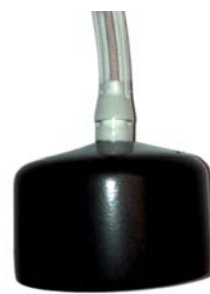
Calibration Cup Assy, IR-RS Cup Inner Diameter: 42.8mm Tubing Inner Diameter: 5mm Note: The cup has four equal cuts to allow it to fit over the IR-RS sensor as shown below. Usage: IP41 units with IR-RS sensor
