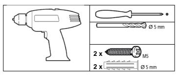
1. To fix the module directly to the wall, use the cut out below to make the 2 holes "B" at the distance indicated in fig. 1.
