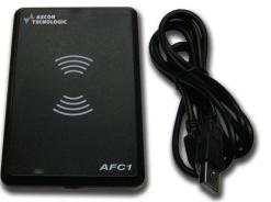
To configure the instrument with the **NFC**, it is not necessary to power the timer, but simply put its front panel on the symbol ((\* )) of the **AFC1** device surface (which is powered directly by the **USB** port connected to the **PC**) or on the smartphone part on the which is the **NFC** interface (for this consult the smartphone user manual) then send the parameters to the instrument's memory.
