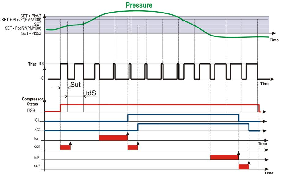
The capacity of the DGS compressor is limited by the PM and PMA parameters, where
